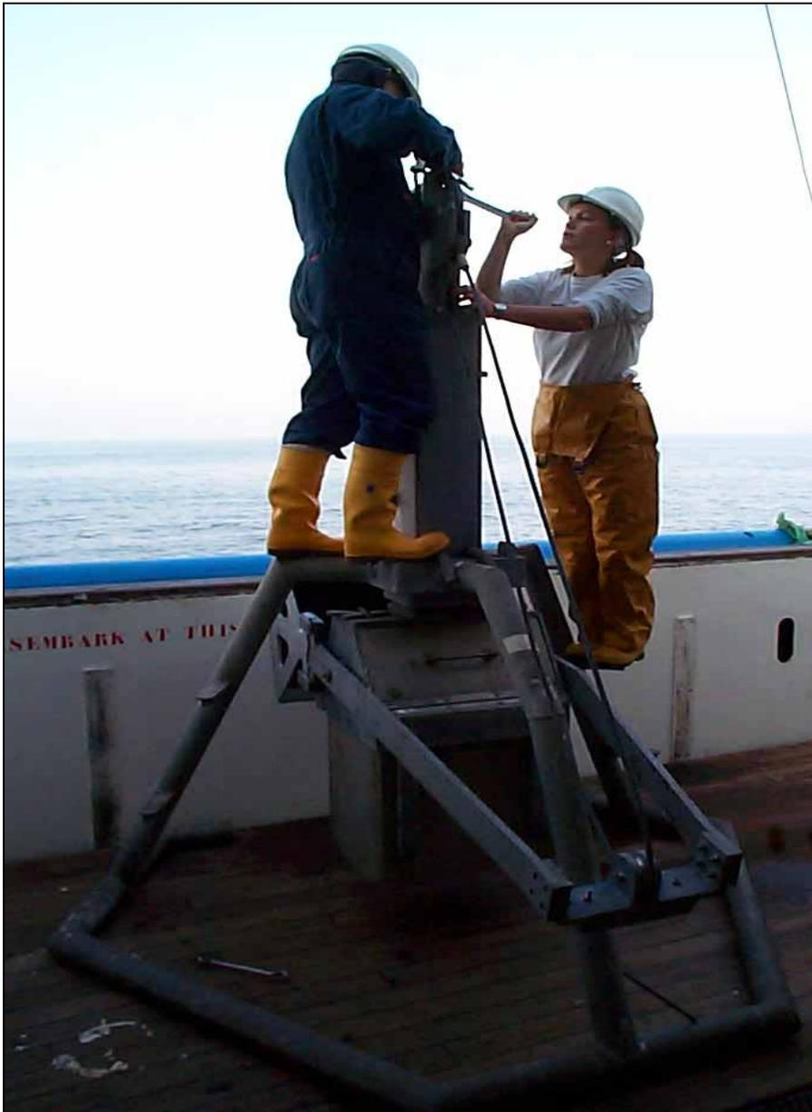
Figure 6.5.21.1. Box corer of FRS Marine Laboratory
